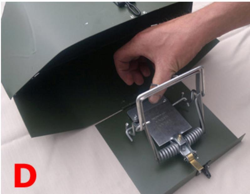
**E** - Place your other thumb over the round wire jaw, ease the jaws apart against the force of the springs. The springs are very strong and it is a good idea to practice opening and closing the jaws slowly to improve technique and gain confidence.
