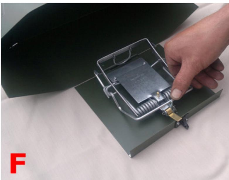
**G** - To set the trap; the brass trigger plate must be turned over the top of the round wire jaw and located within the brass notch on the treadle plate. The jaws will need to be pressed open a little further and the treadle plate raised before the two parts can be engaged.
