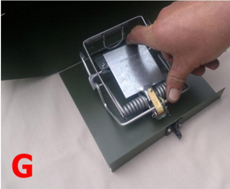
**H** - With the safety catch still in position bait your trap with peanut butter or a bait of your choice, then remove the safety hook from over the jaw. We recommend using a stick or a piece of wire.
