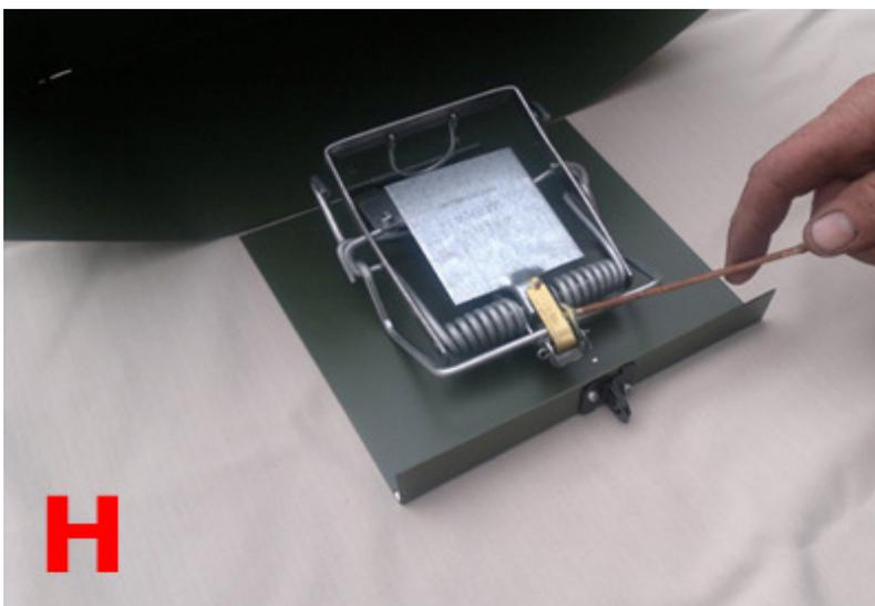
**I** - With the safety catch removed the force of the springs will clamp the jaws together when the squirrel puts pressure on the treadle plate disengaging it from the trigger holding the round wire jaw.
